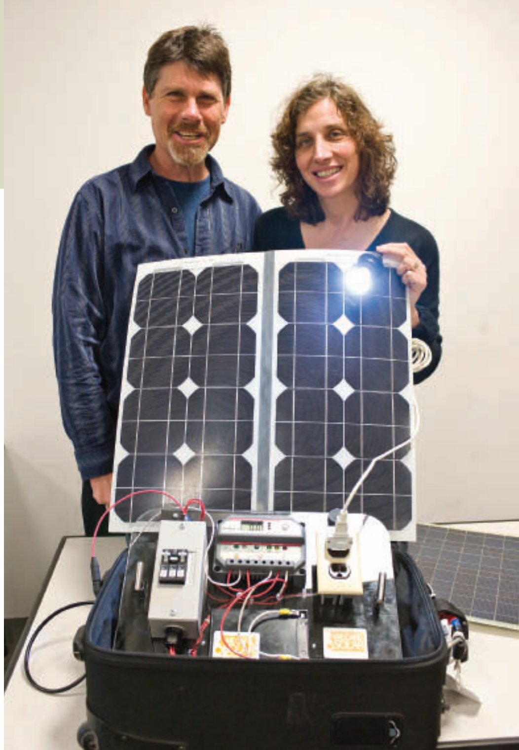
Dr. Hal Aronson and Dr. Laura Stachel, founders of WE CARE Solar, developed a photovoltaic system that powers lighting, mobile communications, and essential medical devices – that fits in a carryon suitcase.
